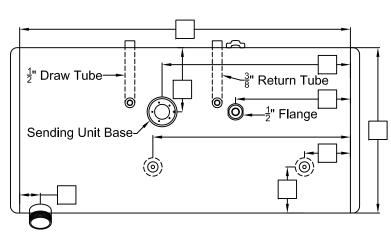
Please note: All sizes are NPTF unless otherwise noted and reference all measurements from the lateral weld seam and the end cap weld seam to the center of the fittings.
